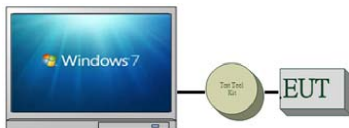
Fig. 2-1 Radiated & Conducted (Antenna Port) Emission Configuration
