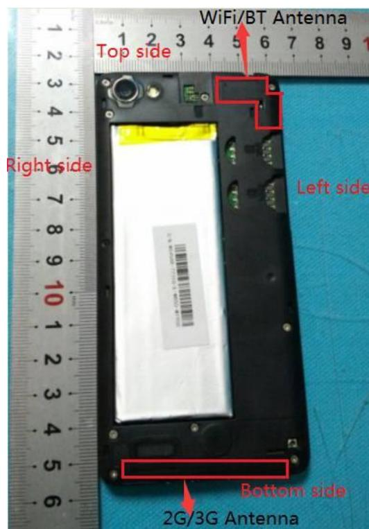
The SAR measurement positions of each side are as below:
