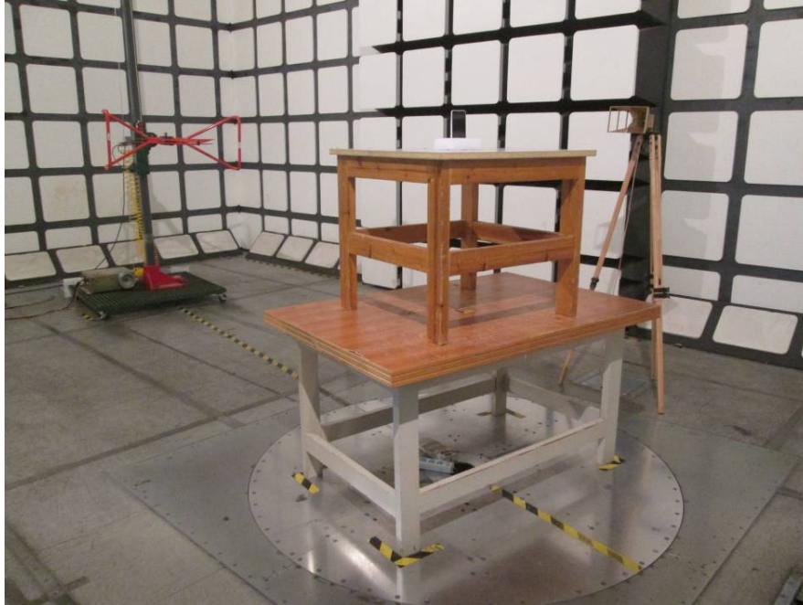
Radiated Emissions Test View (Below 1 GHz)
