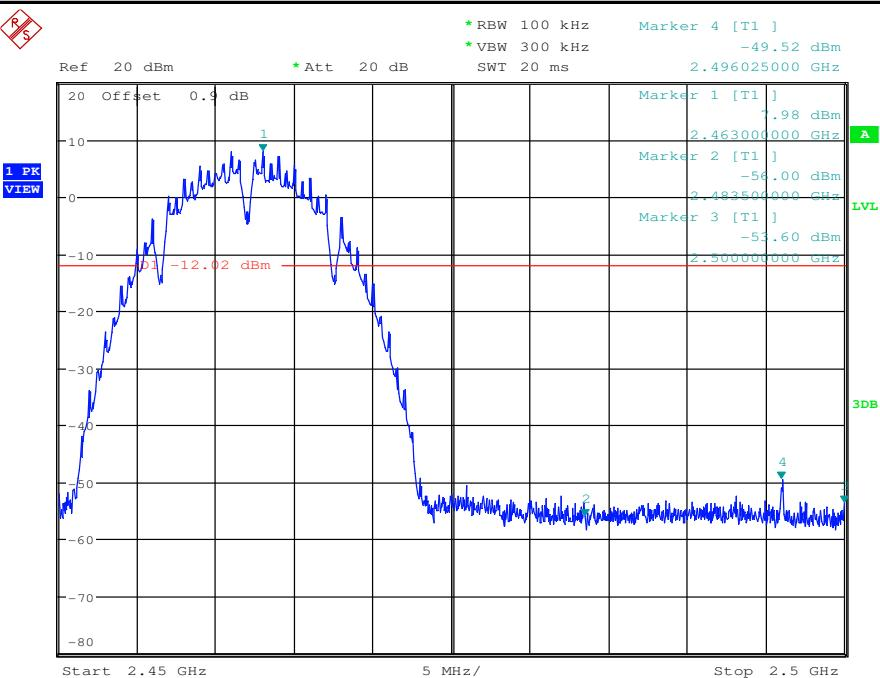
**Band-edge for RF Conducted Emissions\_11B\_2462\_Ant2**
