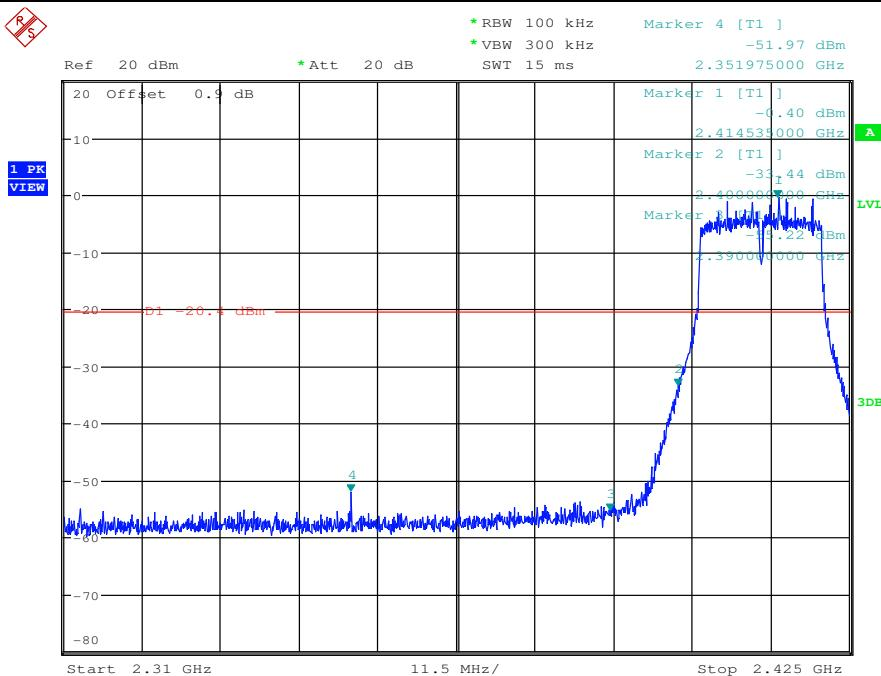
Band-edge for RF Conducted Emissions\_11N20SISO\_2412\_Ant2
