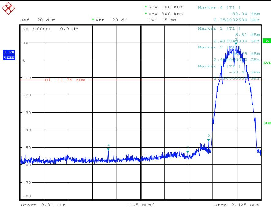
Band-edge for RF Conducted Emissions\_11B\_2412\_Ant2
