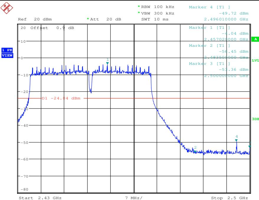
**Band-edge for RF Conducted Emissions\_11N40SISO\_2452\_Ant2**
