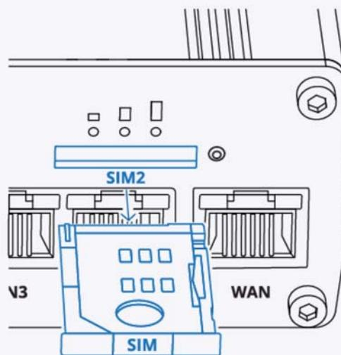
**5. Slide the SIM holder back into the router.**
