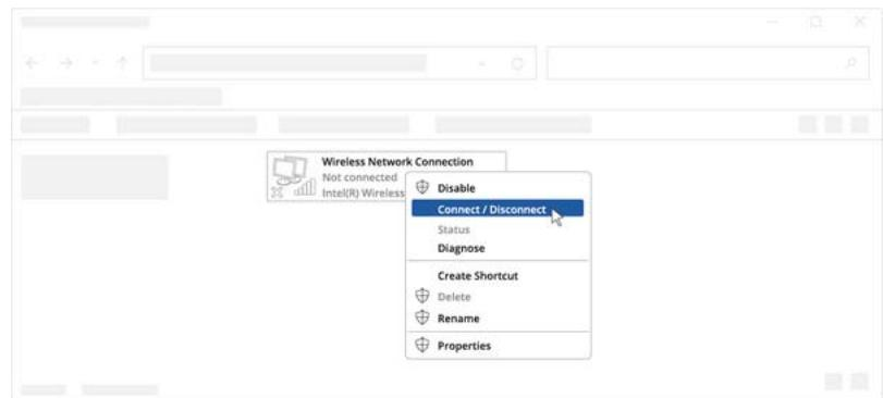
5. Choose the wireless network RUTM54 \*\*\*\* from the list and click Connect. Enter the Wi-Fi password located on the device's label.
