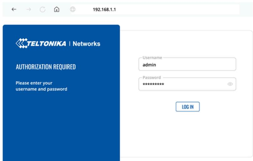
3. After logging in, you must set a new password for security reasons. You will not be able to interact with the router's WebUI until the default password is changed. The new password must consist of a minimum of **8 characters**. Requirements: one uppercase letter, one lowercase letter, and one digit.
