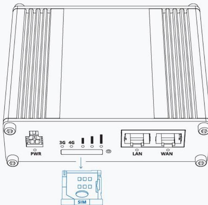
**5. Slide the SIM holder back into the router.**
