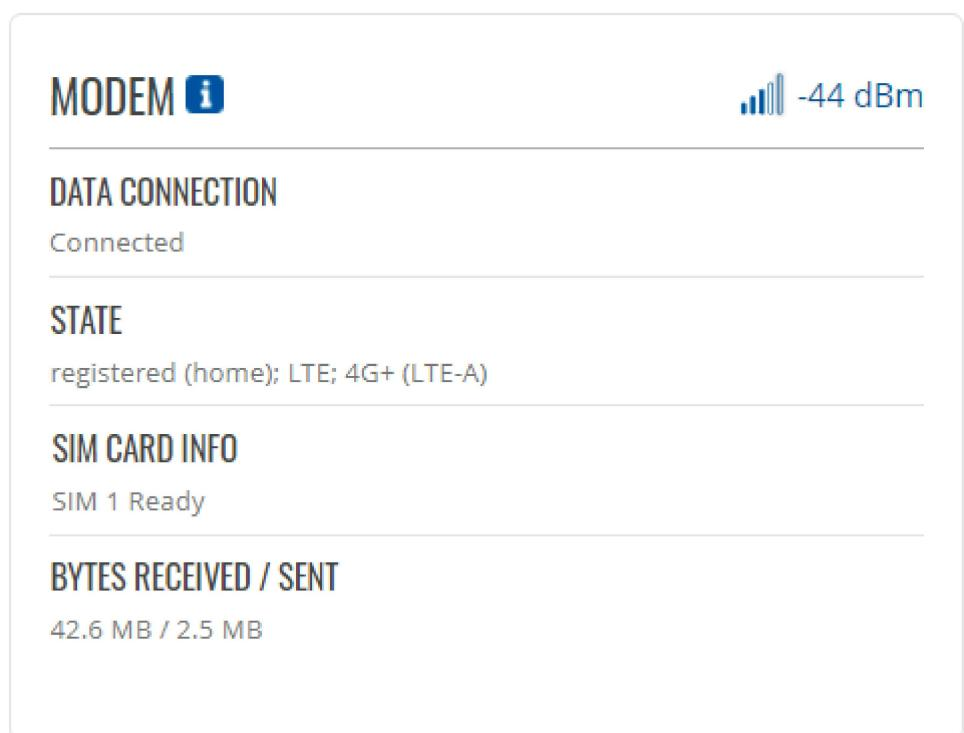
A screenshot of the Teltonika Networks RUT271 Status — Network page. The page has a header with 'MODEM' and signal strength '-44 dBm'. Below this, there are several sections: 'DATA CONNECTION' (Connected), 'STATE' (registered (home); LTE; 4G+ (LTE-A)), 'SIM CARD INFO' (SIM 1 Ready), and 'BYTES RECEIVED / SENT' (42.6 MB / 2.5 MB).
