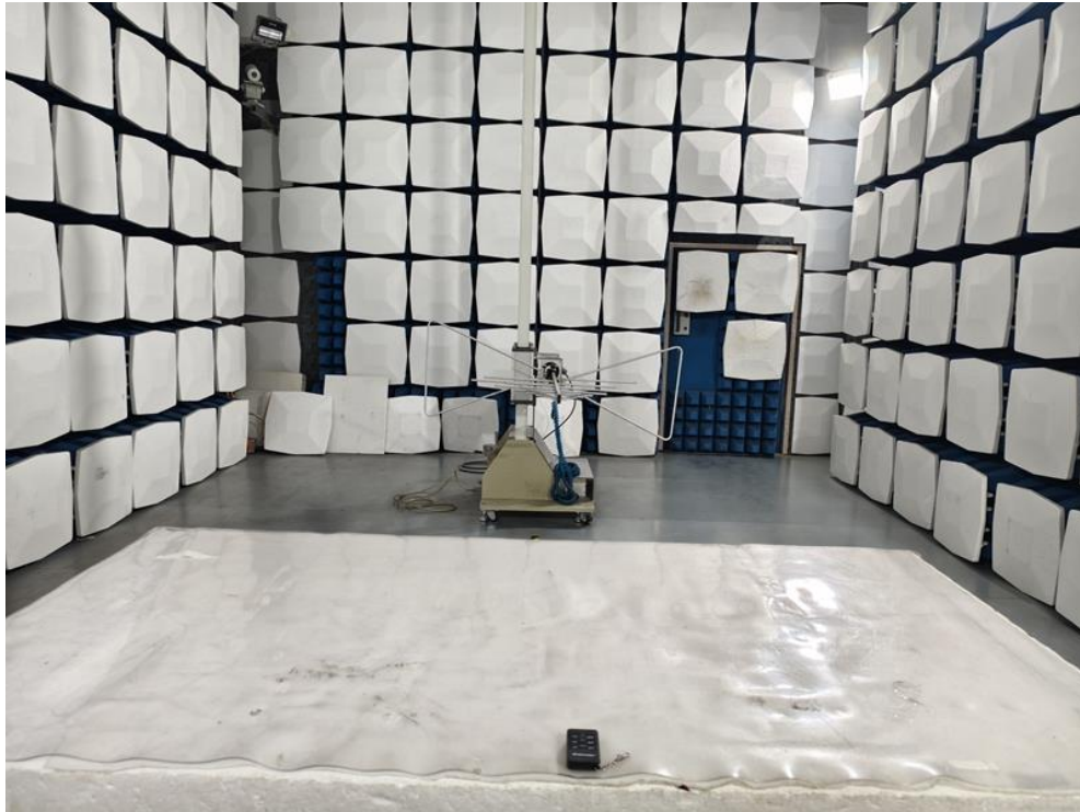
Radiated Emission Test Setup:
