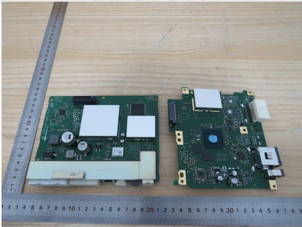
M3GL06R Internal View of EUT-7
