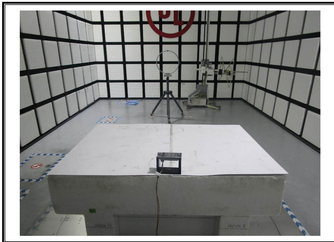
RADIATED EMISSIONS MEASUREMENT SETUP (Below 30MHz)
