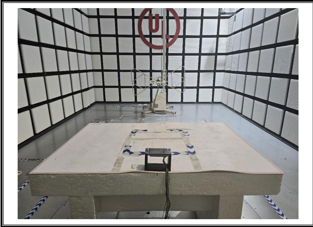
RADIATED EMISSIONS MEASUREMENT SETUP (30MHz ~ 1 GHz)
