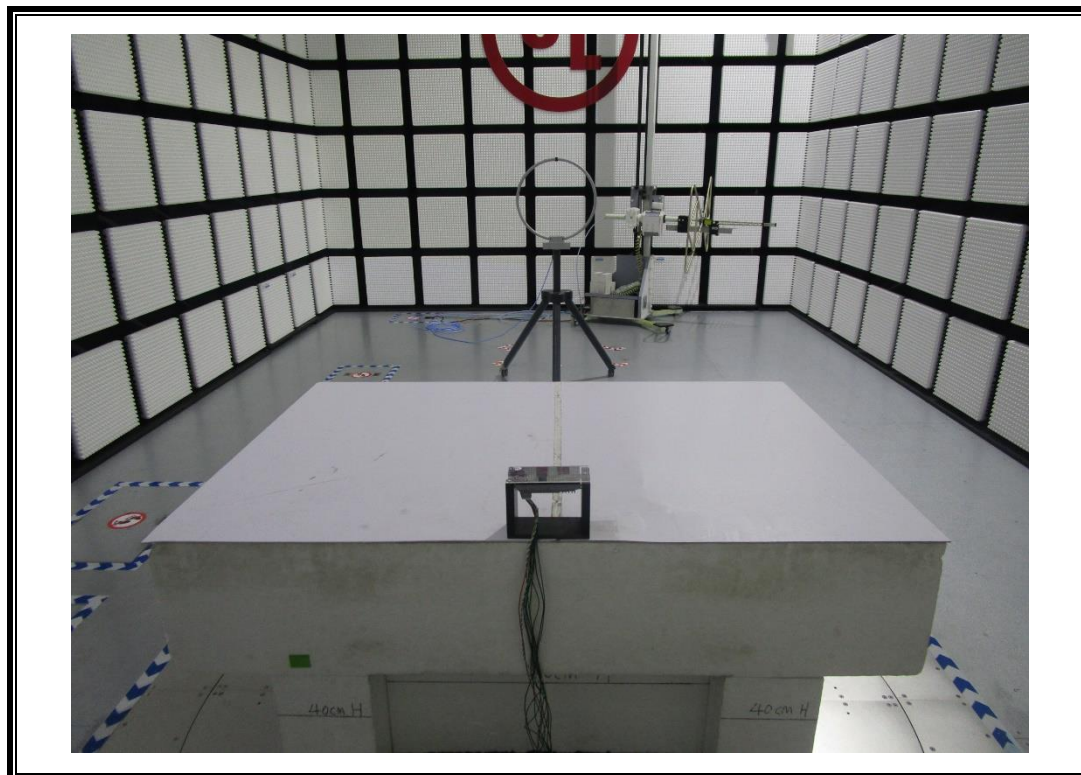
RADIATED EMISSIONS MEASUREMENT SETUP (Below 30MHz)
