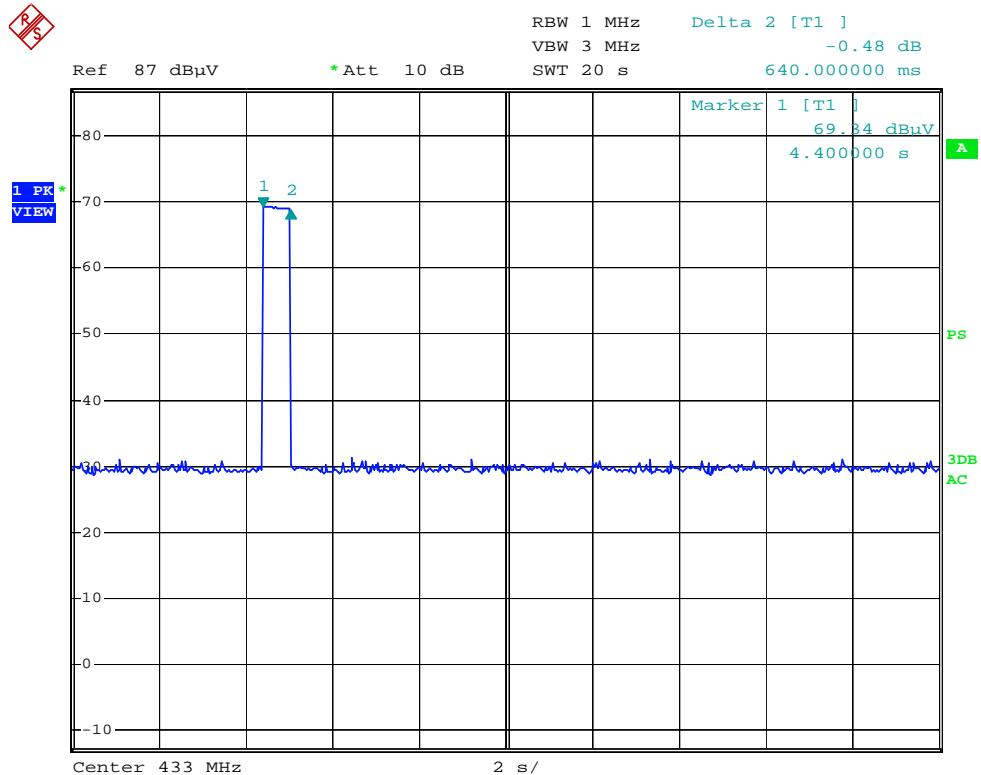
**3. Regulation 15.231 (a2)** A transmitter activated automatically shall cease transmission within 5 seconds after activation.
