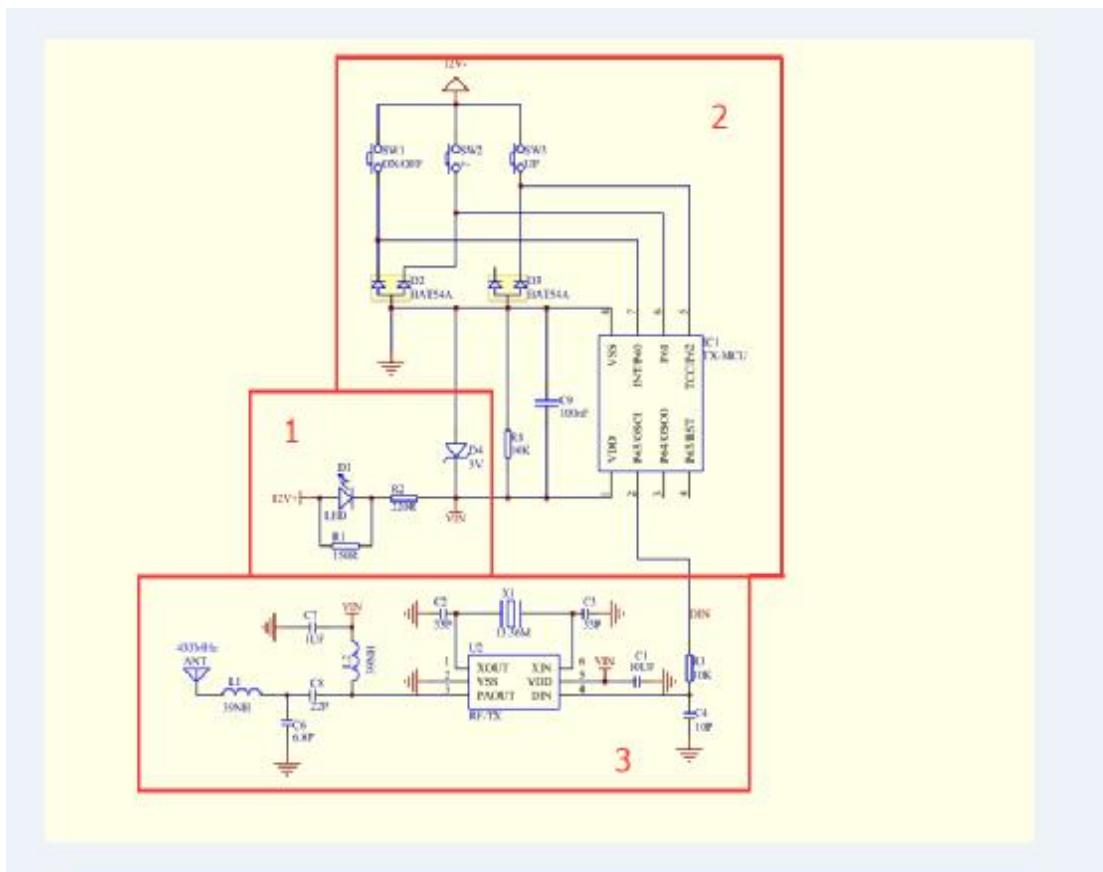
Image 1. 12V battery through LED working Indicator light current-limiting to 3V Regulator circuit
