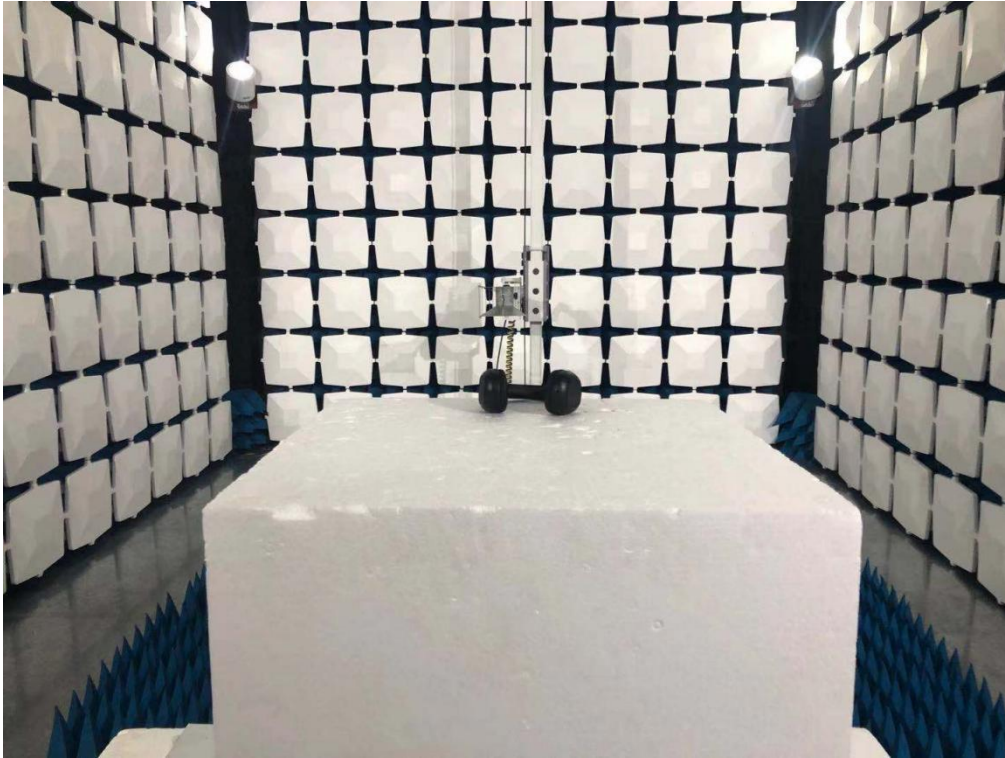
Above 1GHz for radiated emission test setup
