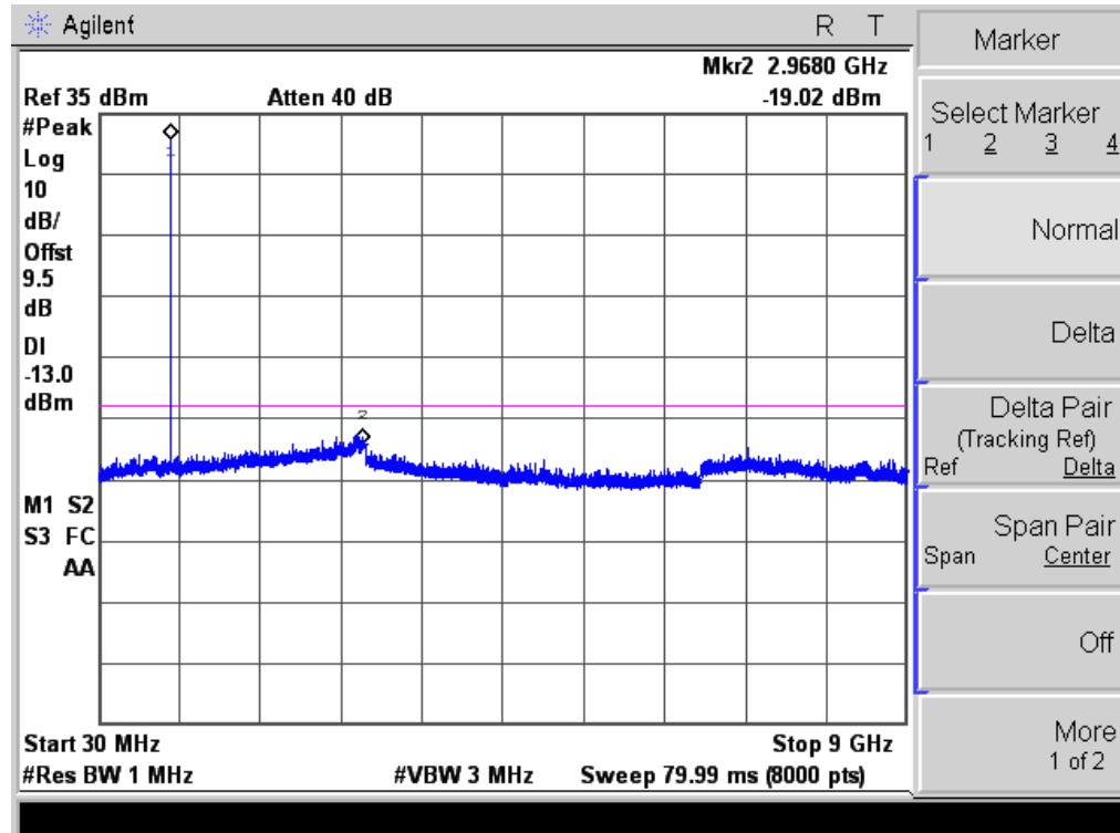
Conducted Emission Transmitting Mode CH 190 30MHz – 9GHz
