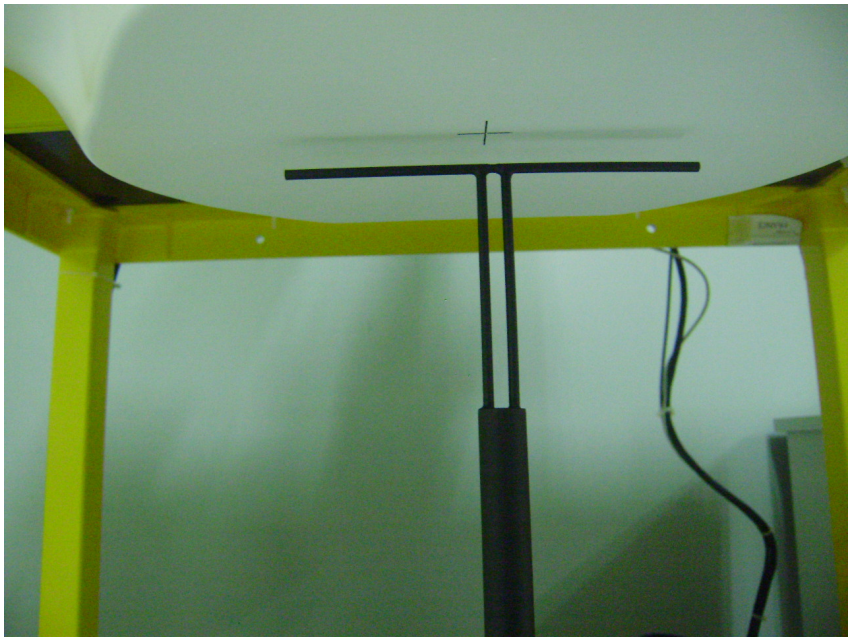
Setup Photo of Dipole Antenna
