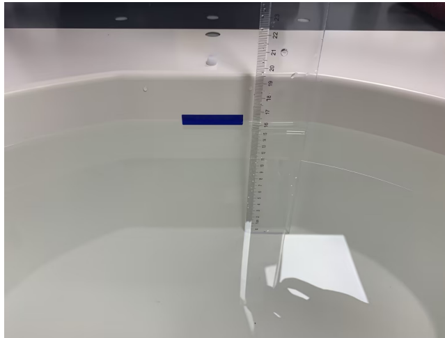
Liquid Height for Head/Body SAR
