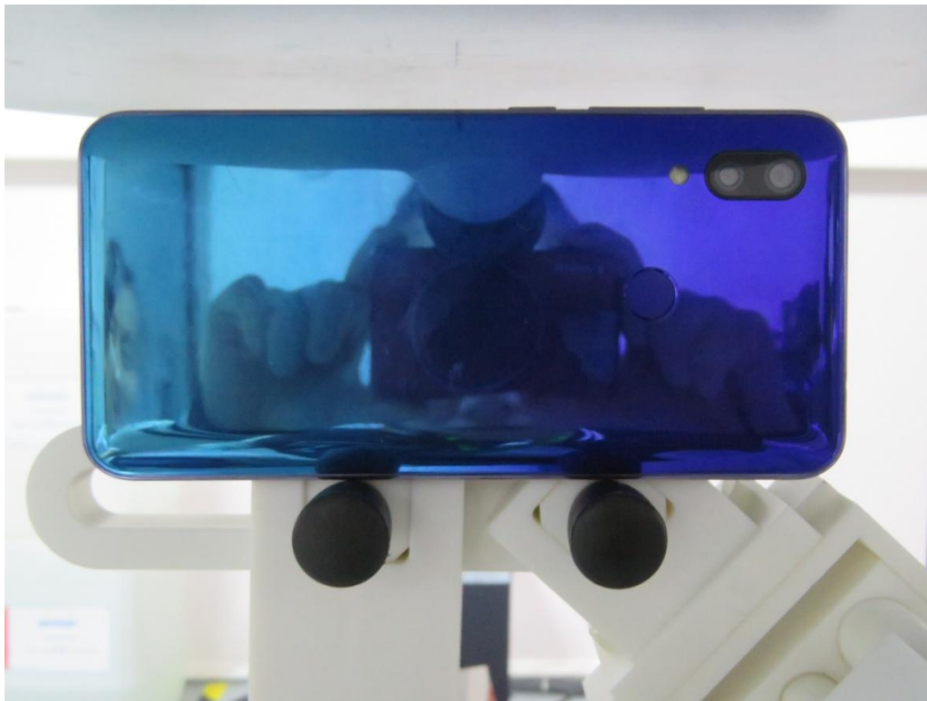
10mm body-worn Right Side Setup Photo (hotspot)
