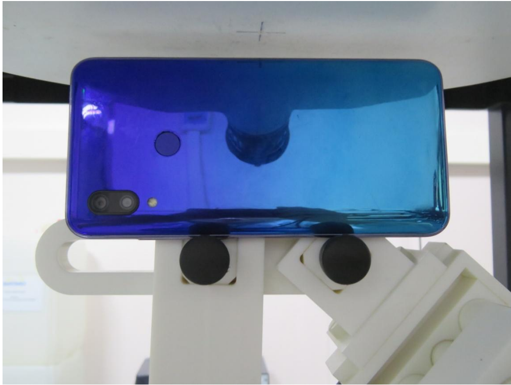
10mm body-worn Left Side Setup Photo (hotspot)
