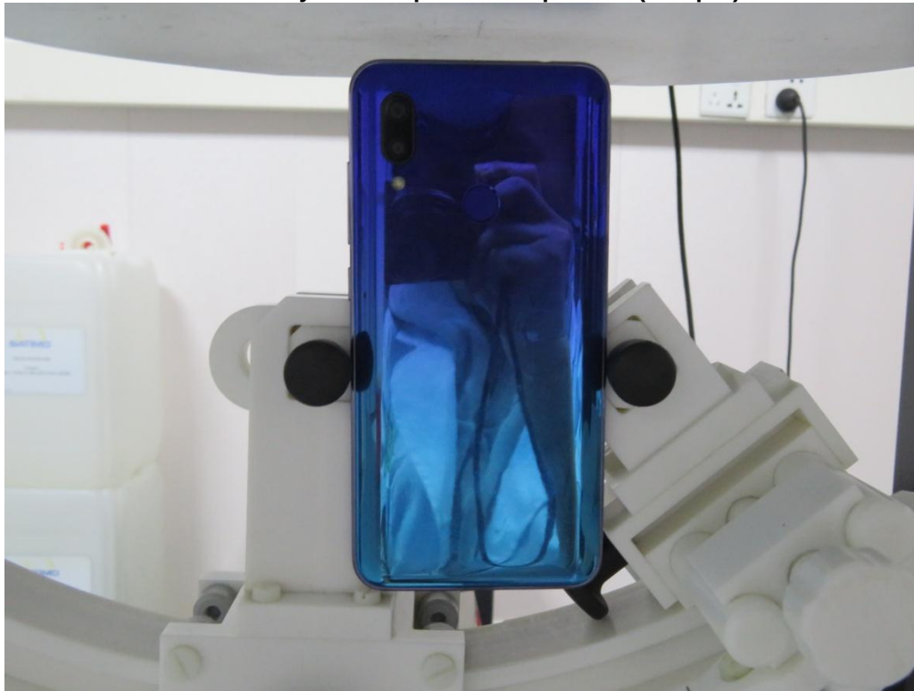
10mm body-worn Top Side Setup Photo (hotspot)
