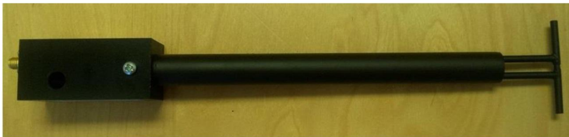
Figure 1 – MVG COMOSAR Validation Dipole
