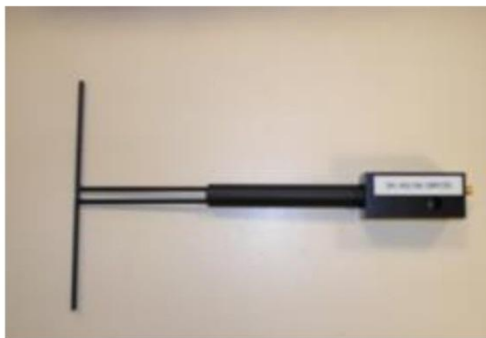
Figure 1 – Satimo COMOSAR Validation Dipole
