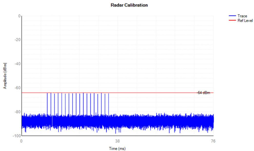
Radar Type 0 (80MHz / 5530Hz)
