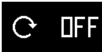
Choose reset icon on the function area, long-pressed 3 seconds to enter the function, click and switch "off" to "on", the system will reset, the time and data will reset to the default value.
