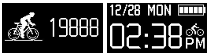
Cycling mode: cycling interface displays calories consumed. Long press key to enter the Ribbon, to record riding time and calories. Riding over long press the button for 3 seconds to return to the menu mode. Riding with the time and the hour record, did not ride without timing.
