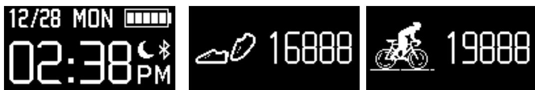
Long press bracelet button for 3 seconds to boot, click the button to switch to display time, date, pedometer, meter, calories, missed call/SMS, sleep time.
