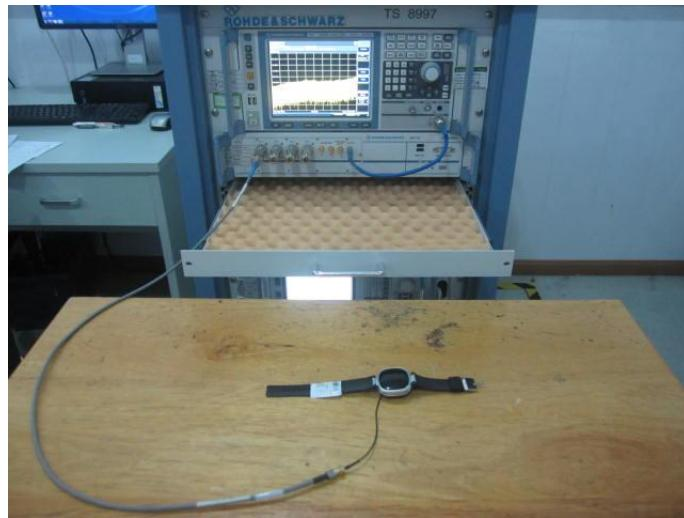
Radiated Emission (9kHz-30MHz)
