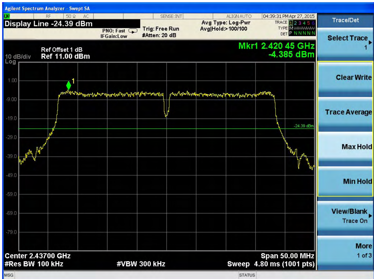
(Plot 4.7.4 B1: Channel 6: 2437MHz @ 802.11n HT40)
