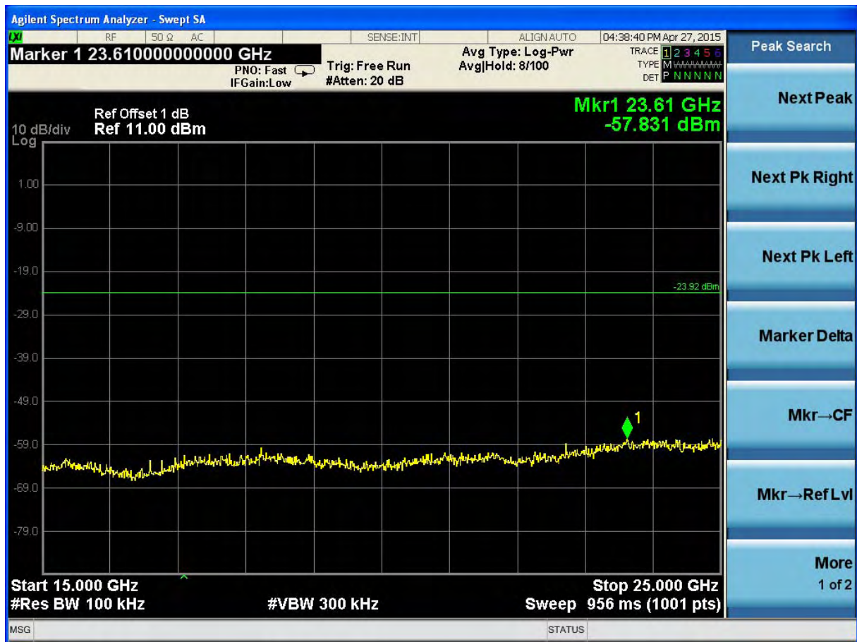
(Plot 4.7.4 A5: Channel 3: 2422MHz @ 802.11n HT40)
