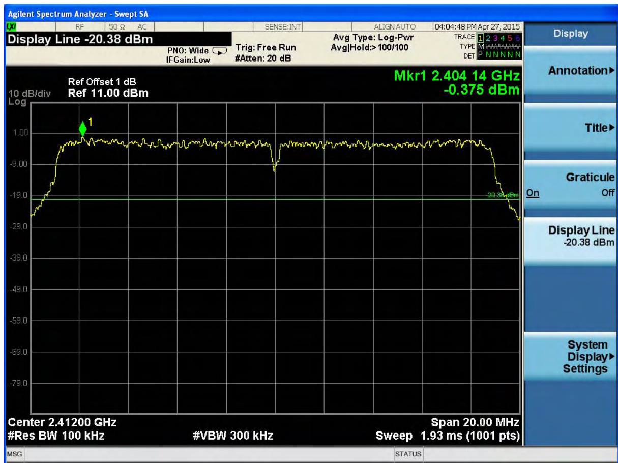
(Plot 4.7.3 A1: Channel 1: 2412MHz @ 802.11n HT20)
