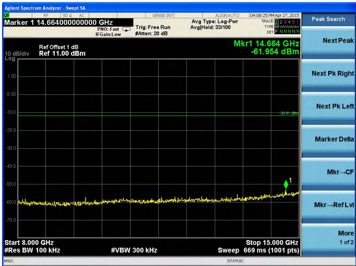
(Plot 4.7.3 B4: Channel 6: 2437MHz @ 802.11n HT20)
