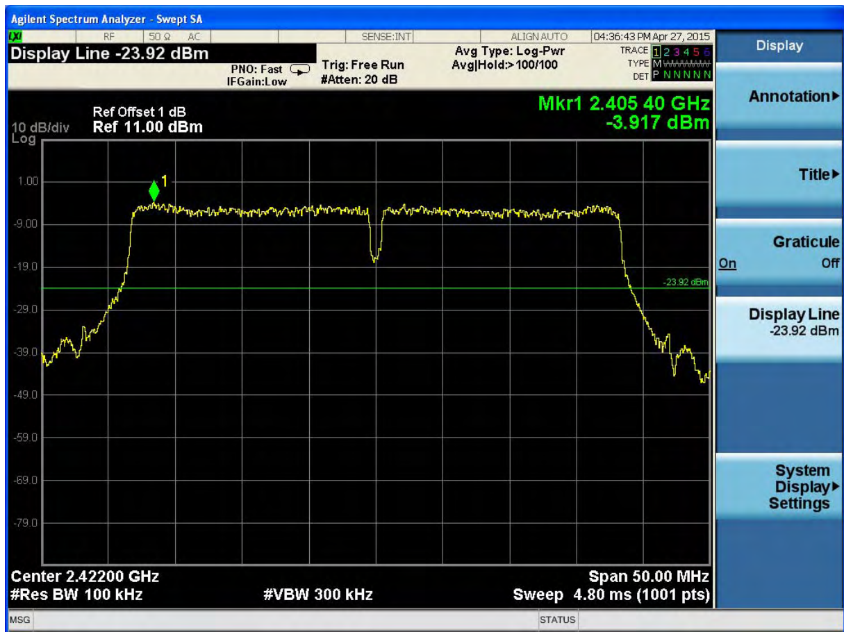
(Plot 4.7.4 A1: Channel 3: 2422MHz @ 802.11n HT40)
