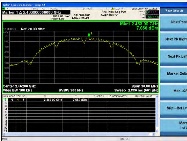
802.11b HIGH CHANNEL, CARRIER LEVEL
