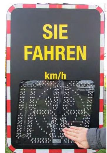
Repeat these steps until your desired threshold value is reached. If you do not make any changes for approx. 10 seconds, the selected safety threshold is confirmed by flashing three times. The start sequence is now continued and ends with the display of the battery voltage. The DSD is ready for operation with the desired threshold value.
