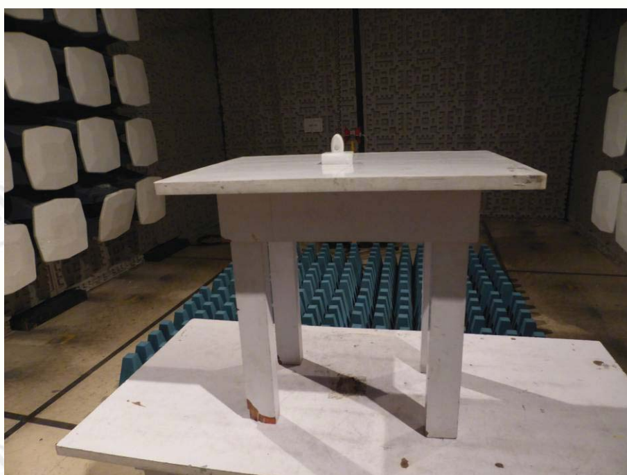
TEST SETUP OF RADIATED EMISSION (above 1GHz)
