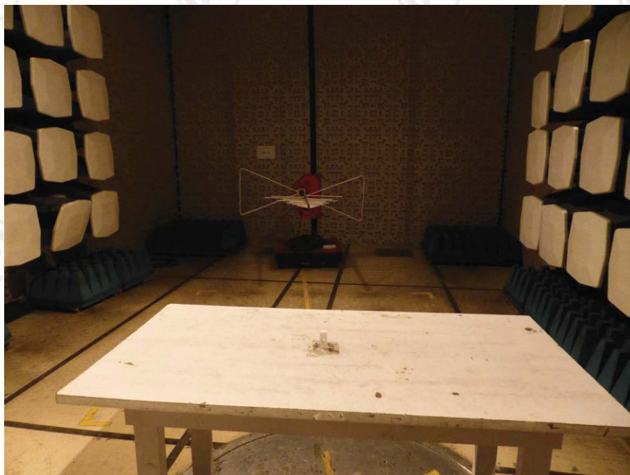
TEST SETUP OF RADIATED EMISSION (30MHz-1GHz)
