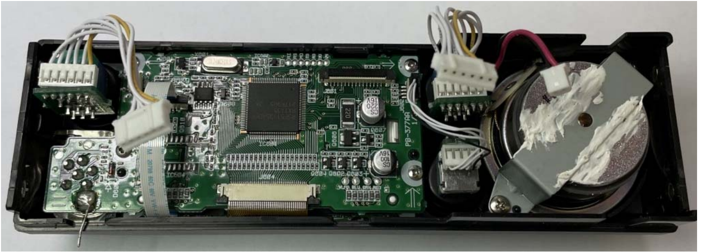
Figure E22.6 – Internal, Main PCB, Front Assembly
