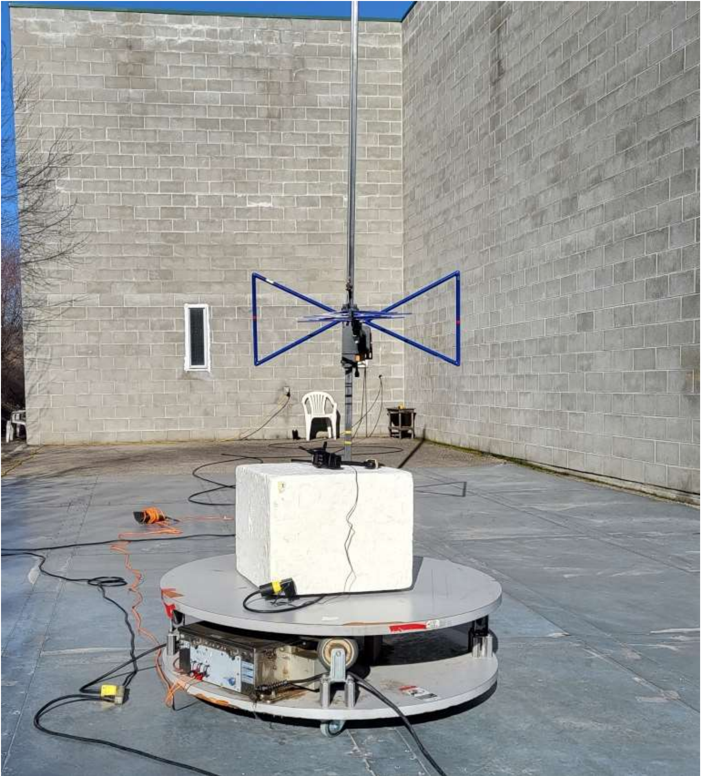
Figure E18.5 – Setup, Radiated Emissions 30 - 1000MHz
