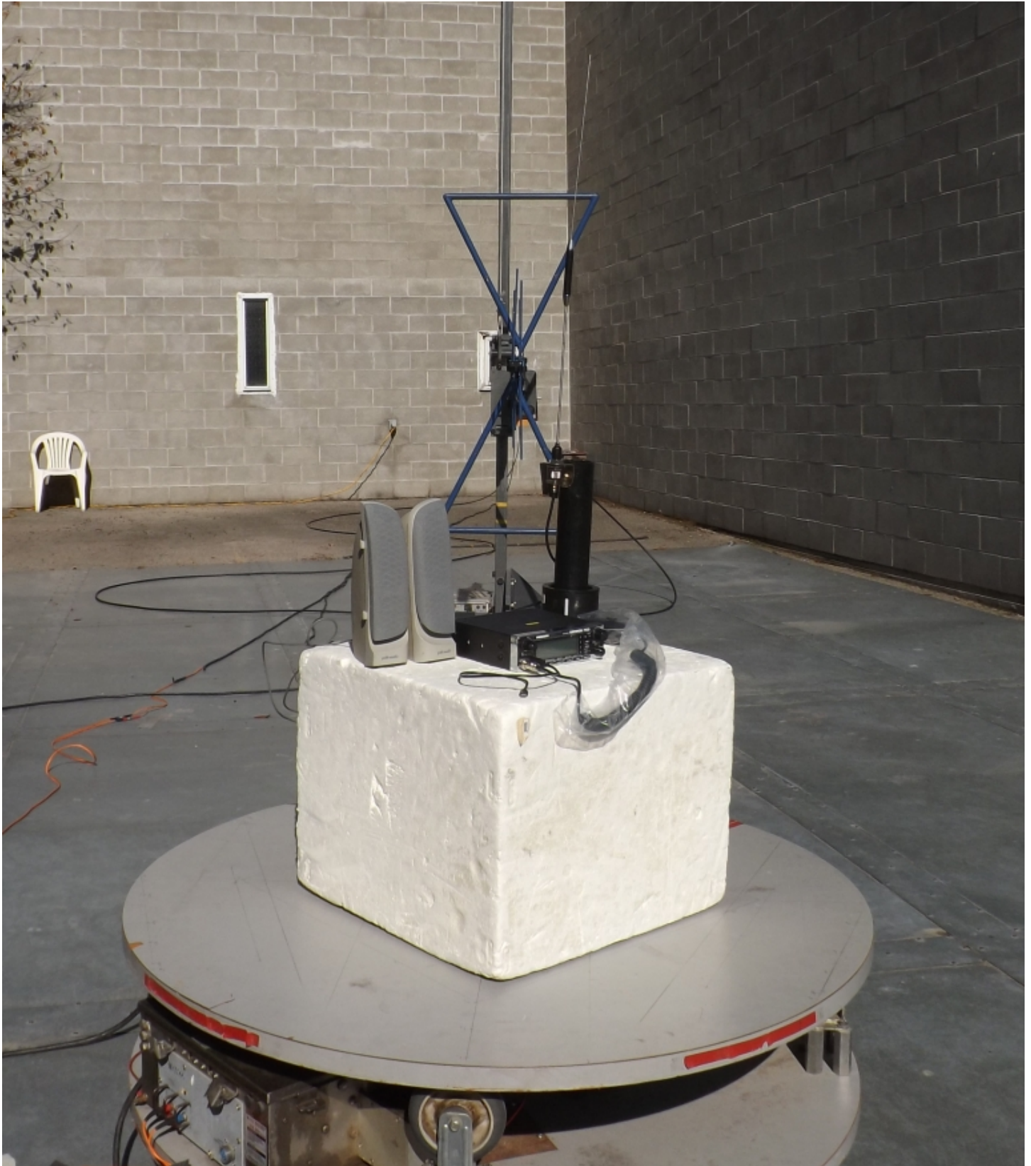
Figure E18.8 – Setup, Radiated Measurements, 30 - 1000MHz, with DUT Accessories
