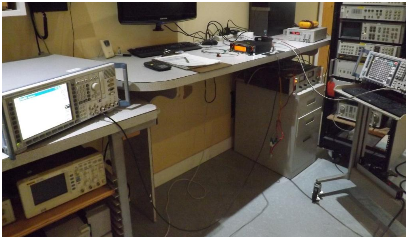
Figure E18.3 – Setup, Single Side Band Measurements with 2-Tone Audio Input
