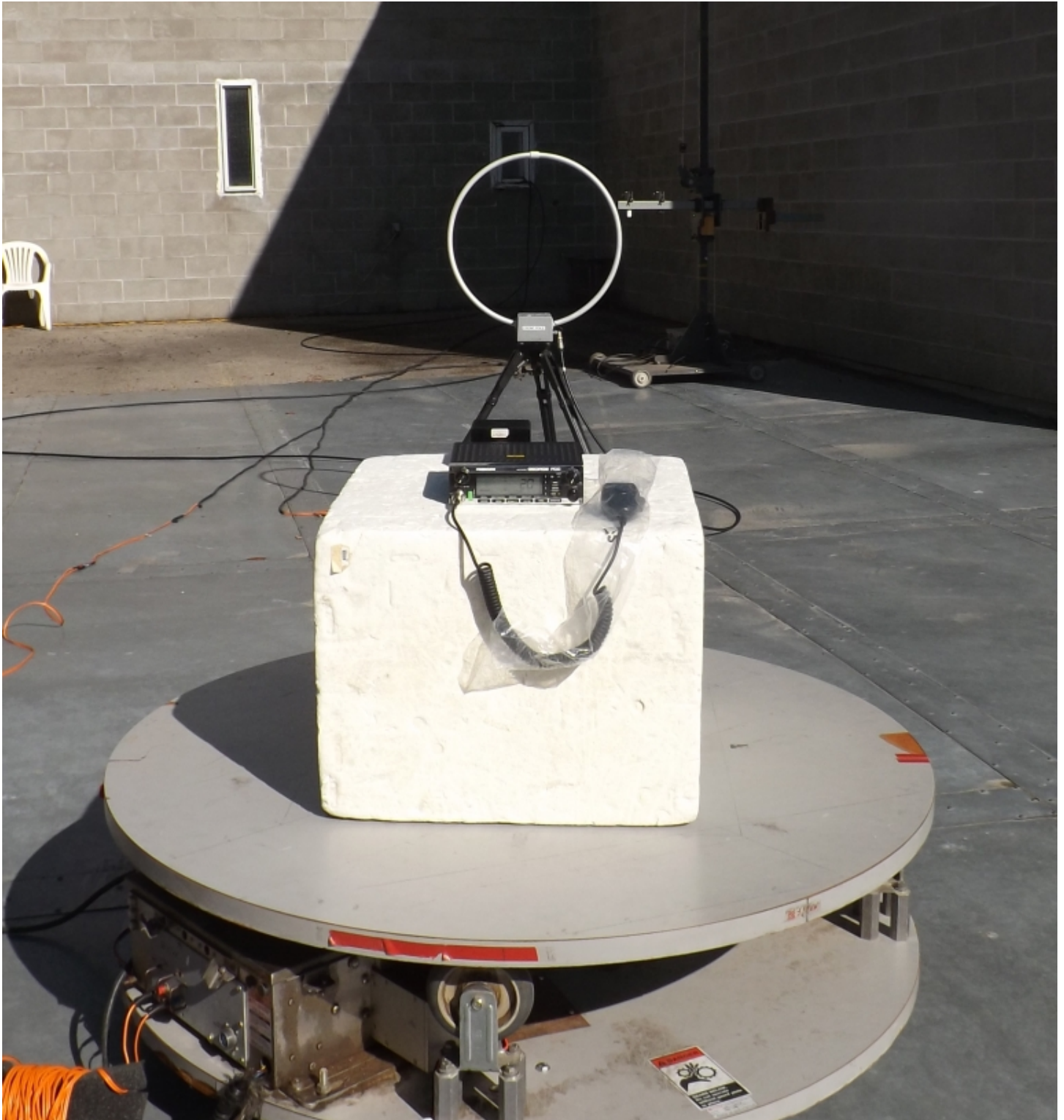
Figure E18.4 – Setup, Radiated Measurements Below 30MHz
