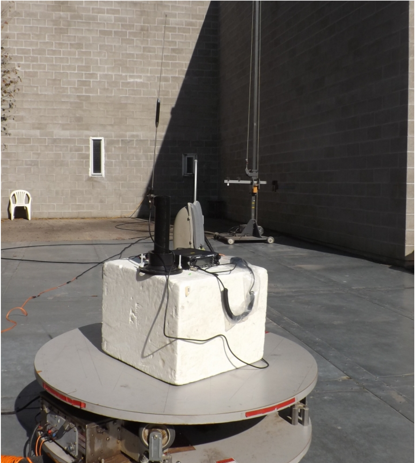
Figure E18.5 – Setup, Radiated Measurements Below 30MHz with DUT Accessories
