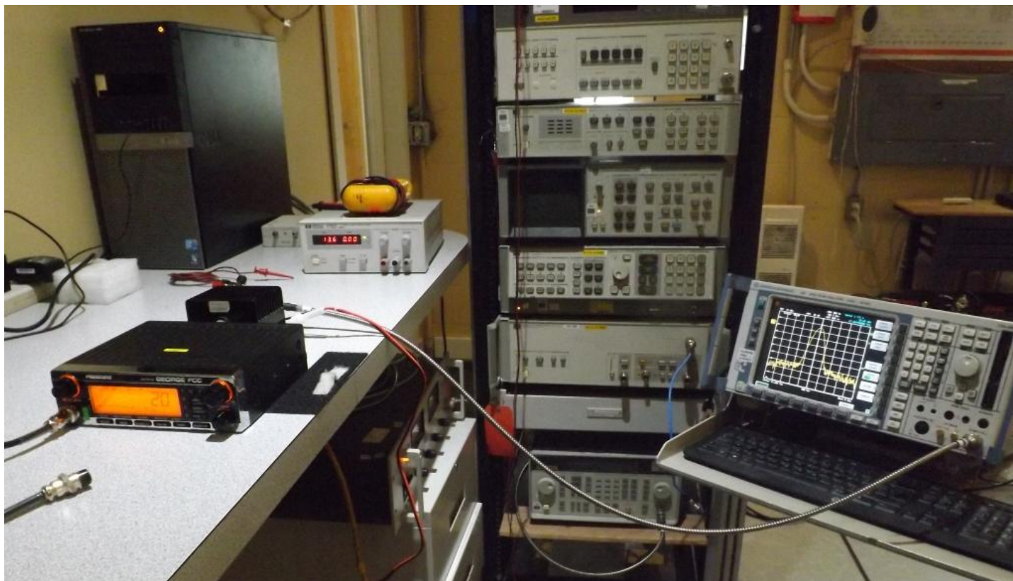
Figure E18.1 – Setup, Antenna Port Conducted
