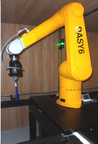
DASY 6 SAR System with SAM Phantom
