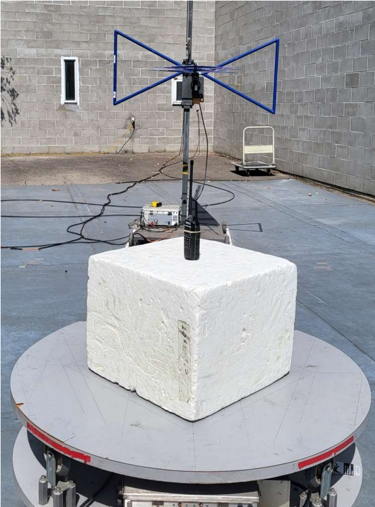
Figure E13.2 – Setup, Radiated Emissions
