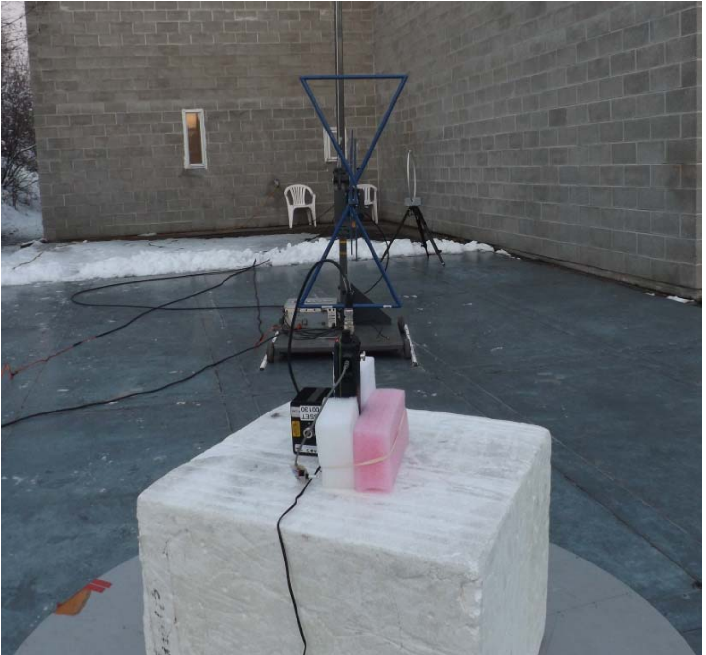
Figure E19.8 – Setup Photo – Radiated Emissions 30 - 1000MHz, Vertical, Without Accessories
