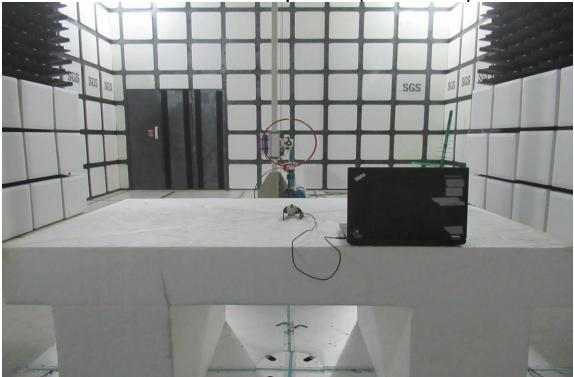
Radiated Emission Setup Photos (30MHz~1GHz)
