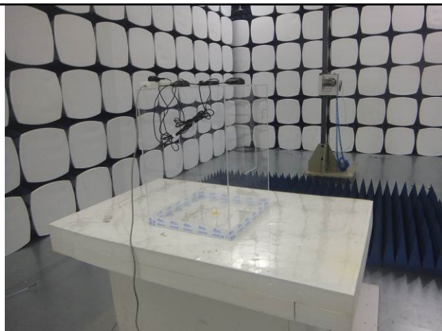
Radiated Spurious Emissions Test Setup Above 1GHz
