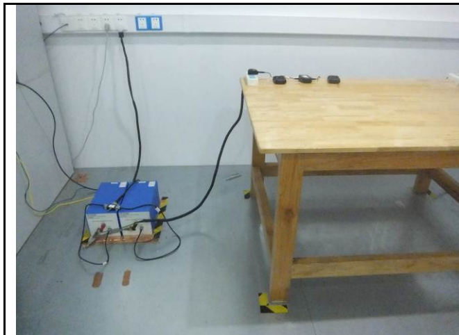
Conducted Emissions Test Setup Front View
