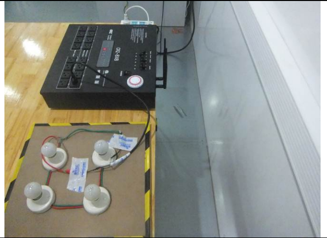
Conducted Emissions Test Setup Side View
