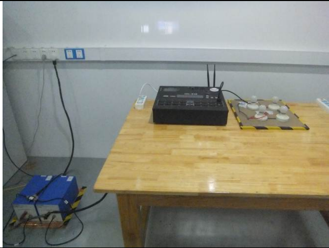
Conducted Emissions Test Setup Front View
