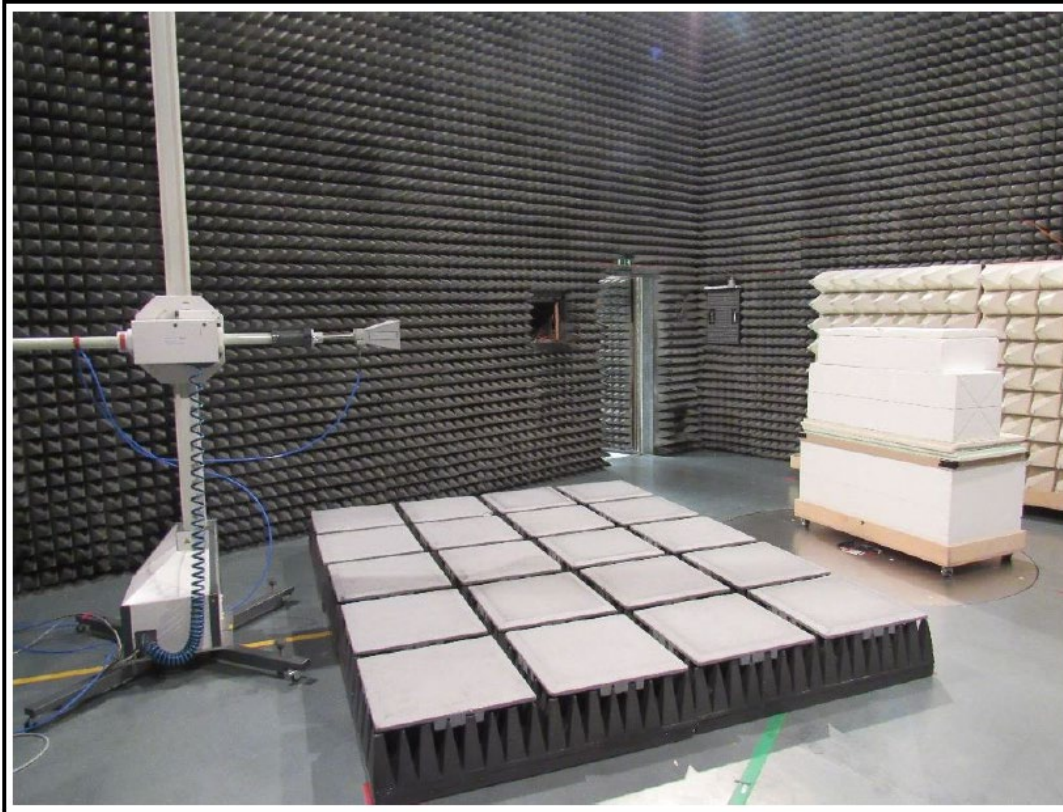
Setup for measurements above 1 GHz
