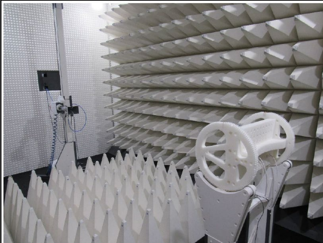
Setup for measurements above 1 GHz
