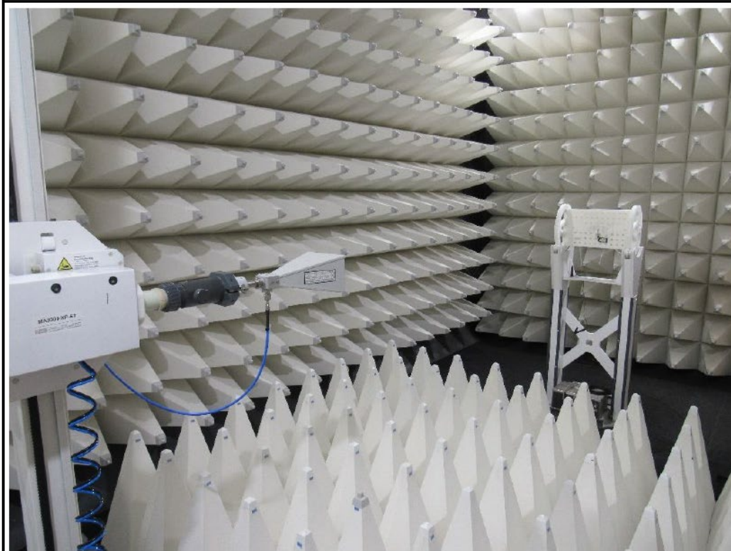
Setup for measurements above 1 GHz
