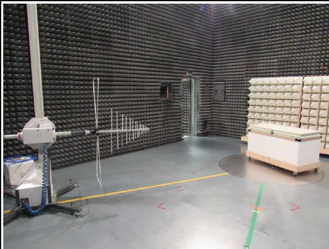
Setup for measurements below 1 GHz
