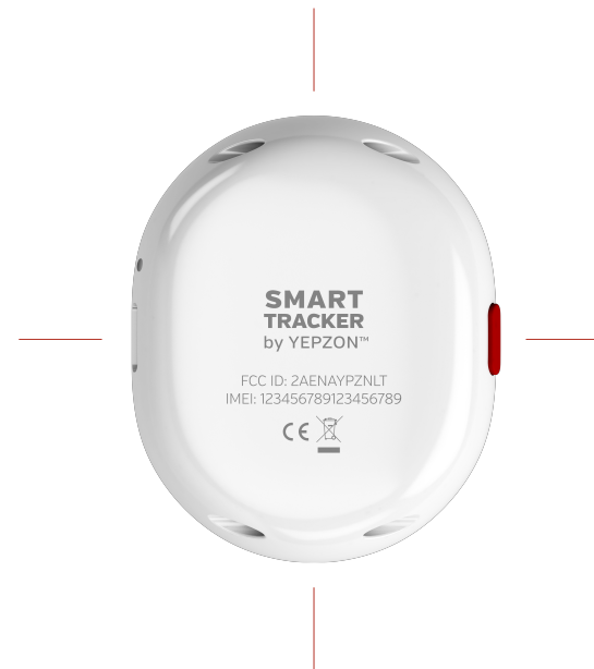
Visualization of laser marked cover
