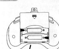
Use screwdriver to loosen the screw and open the battery cover as the arrow direction indicated.
