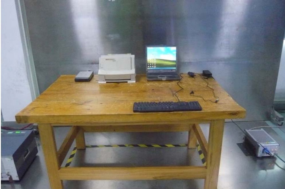
Conducted Emissions – Front View
