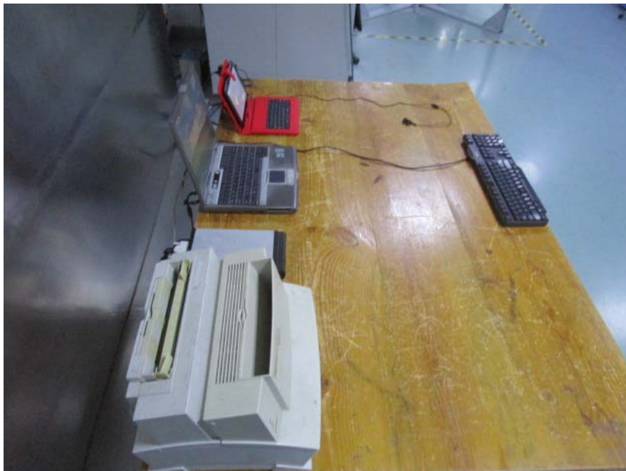
Conducted Emissions - Side View (Charging&Downloading)
