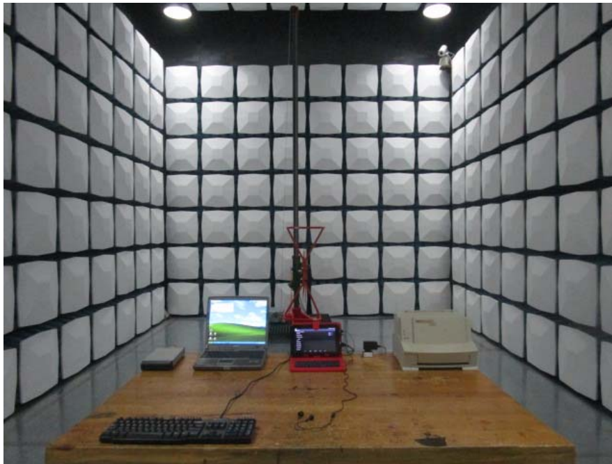
Radiated Emissions –Front View (Below 1GHz) (Charging&Downloading)
