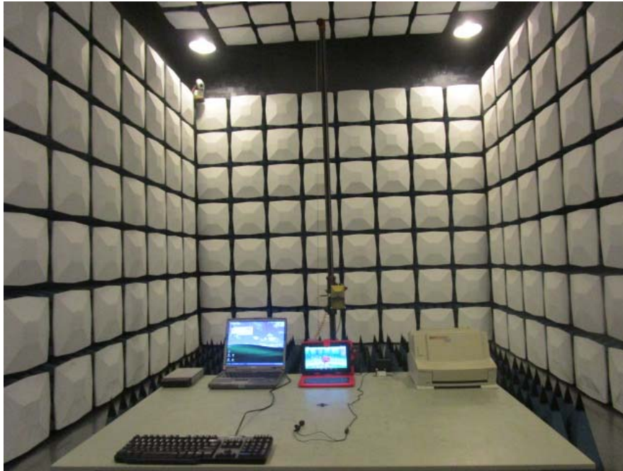
Radiated Emission –Front View (Above 1 GHz) (Charging&Downloading)
