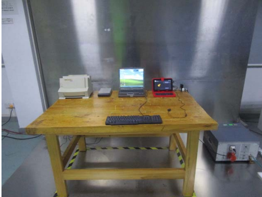
Conducted Emissions – Front View (Charging&Downloading)
