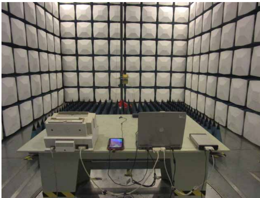
Radiated Emission –Rear View (Above 1 GHz)
