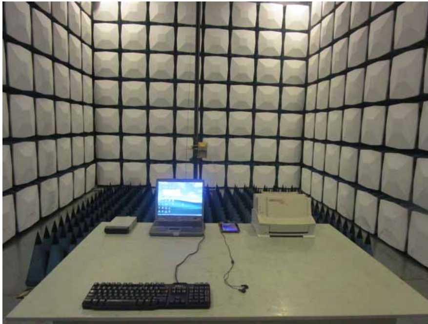
Radiated Emission –Front View (Above 1 GHz)
