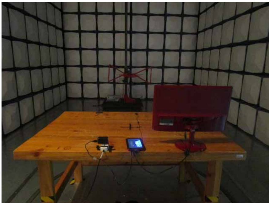
Radiated Emissions –Rear View (Below 1GHz)
