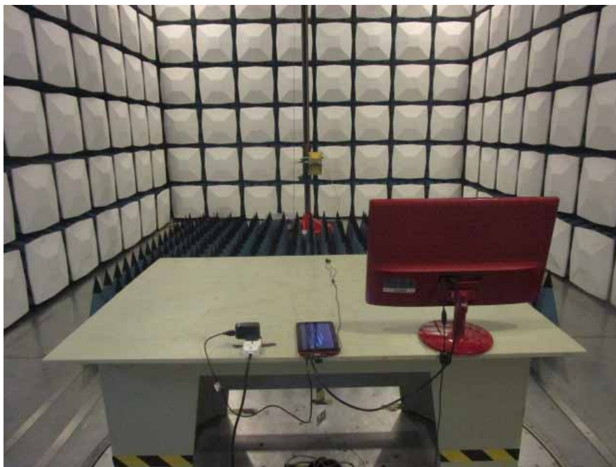
Radiated Emission –Rear View (Above 1 GHz)
