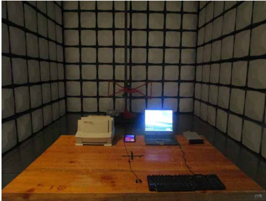
Radiated Emissions –Rear View (Below 1GHz)
