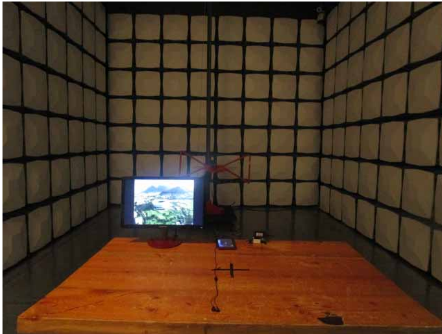
Radiated Emissions –Front View (Below 1GHz)
