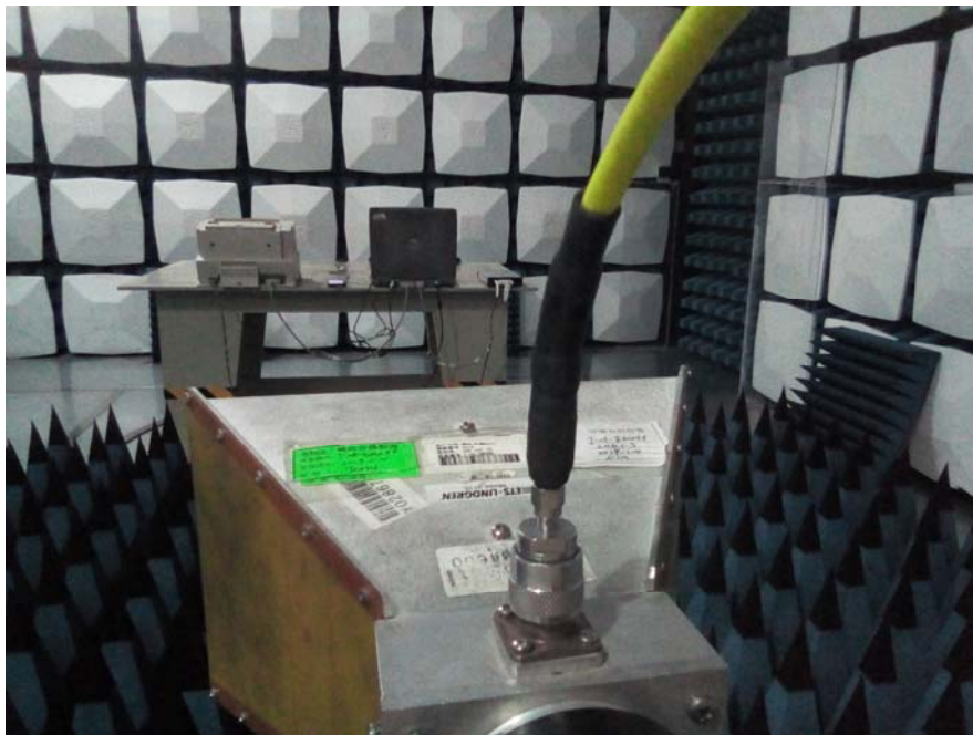
Radiated Emission Above 1GHz – Rear View
