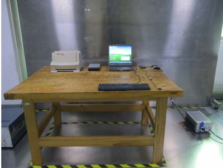
Conducted Emissions – Front View
