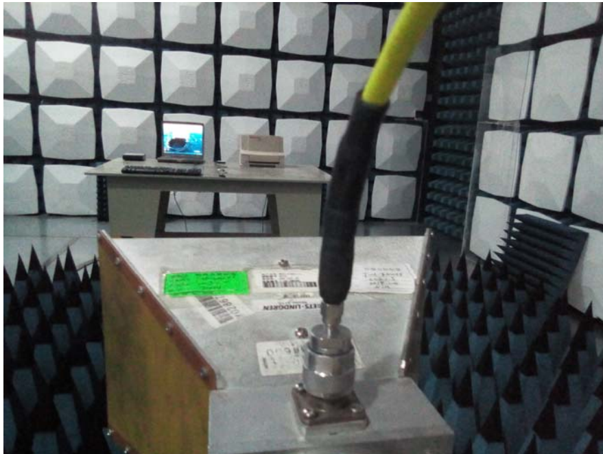
Radiated Emission Above 1GHz – Front View
