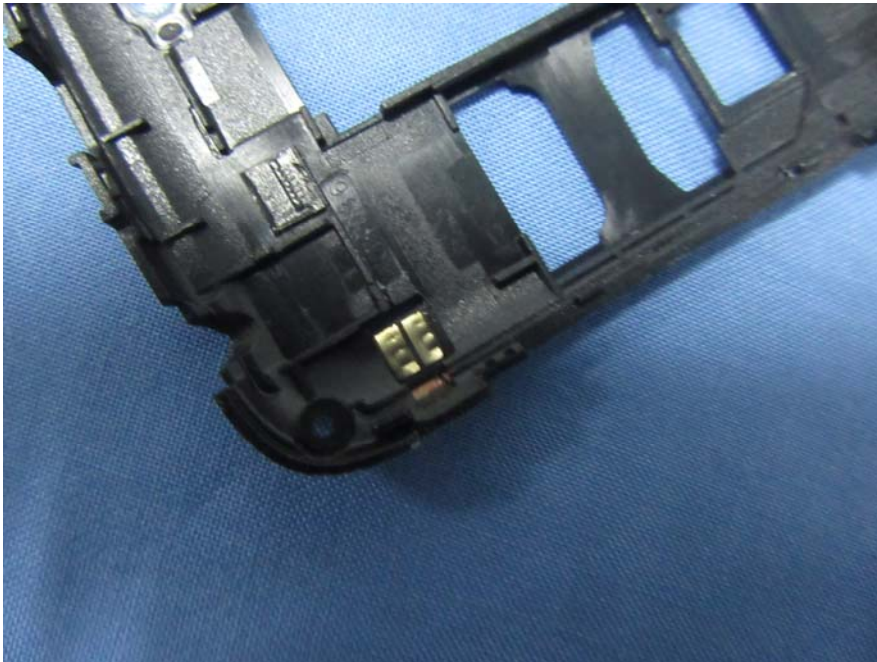
EUT – BT Antenna View
