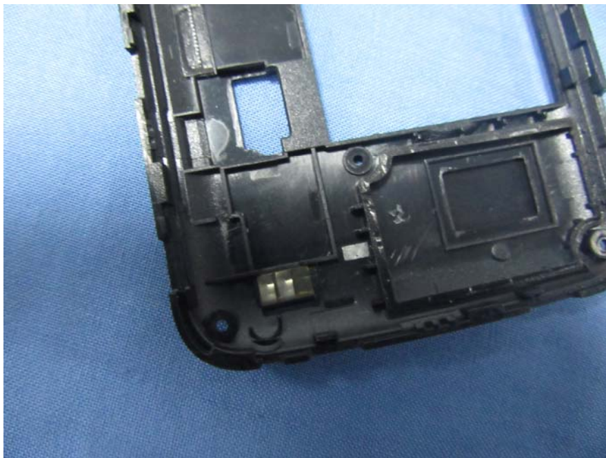
EUT – GSM Antenna View
