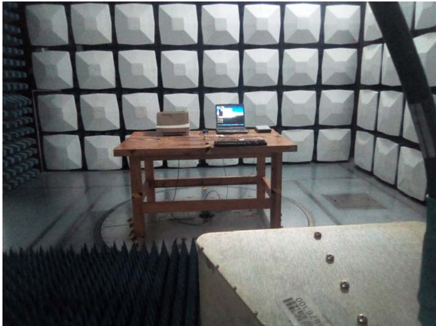
Radiated Emission Above 1GHz – Front View
