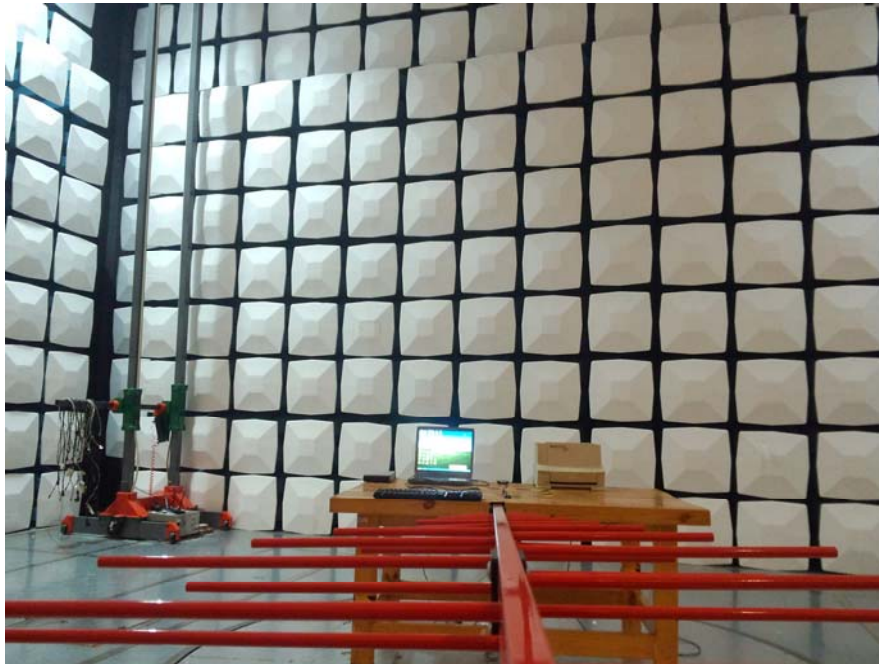
Radiated Emission Below 1GHz – Front View
