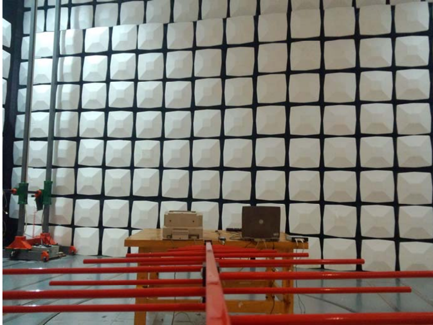
Radiated Emission Below 1GHz – Rear View
