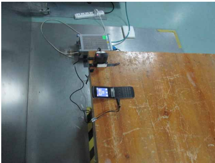
Conducted Emissions – Side View
