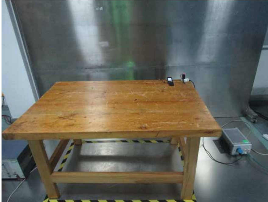
Conducted Emissions - Front View
