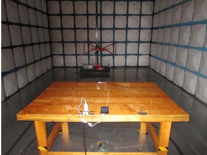
Radiated Emission - Rear View (Below 1GHz)
