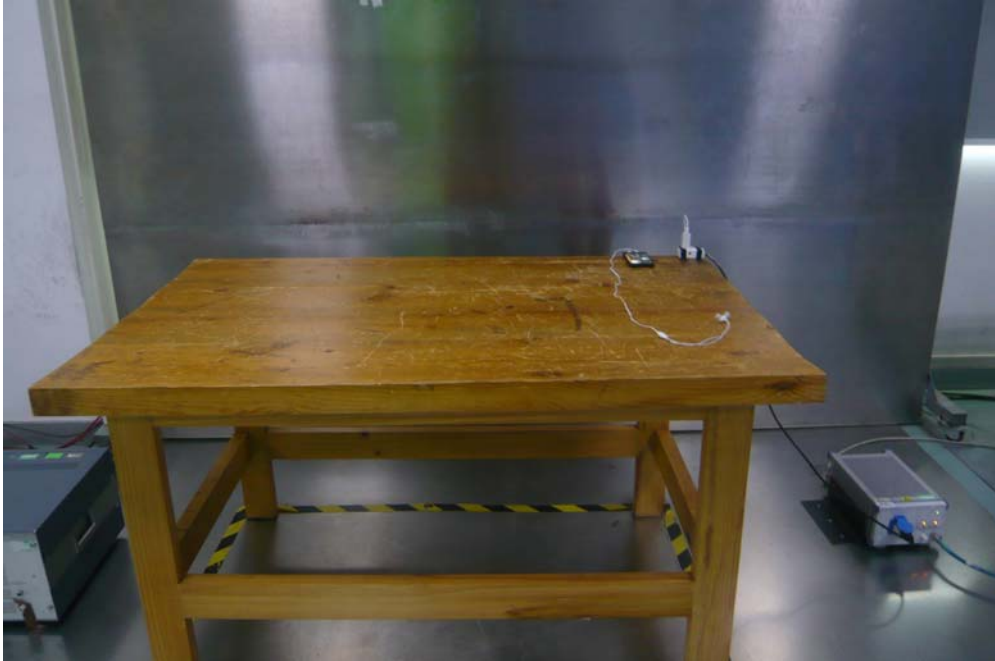
Conducted Emissions – Front View
