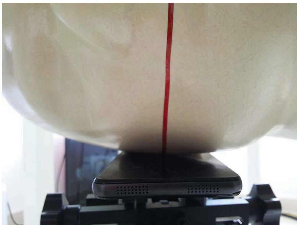
Right Head Cheek Setup Photo
