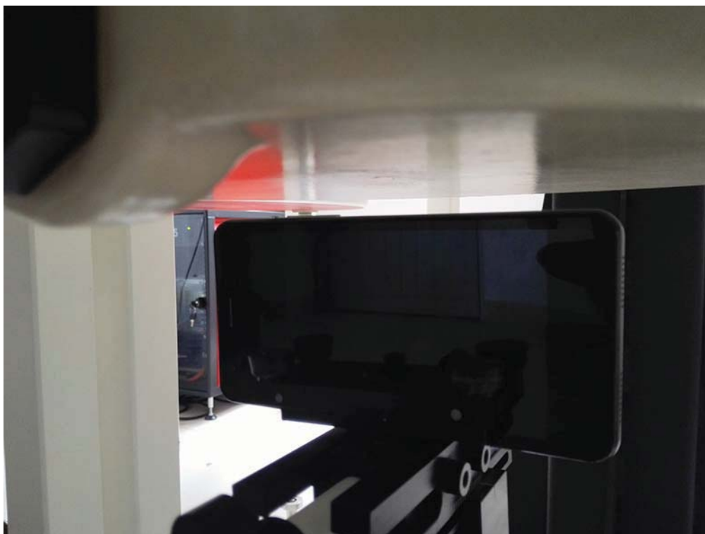
10mm Hotspot mode Right Side Setup Photo
