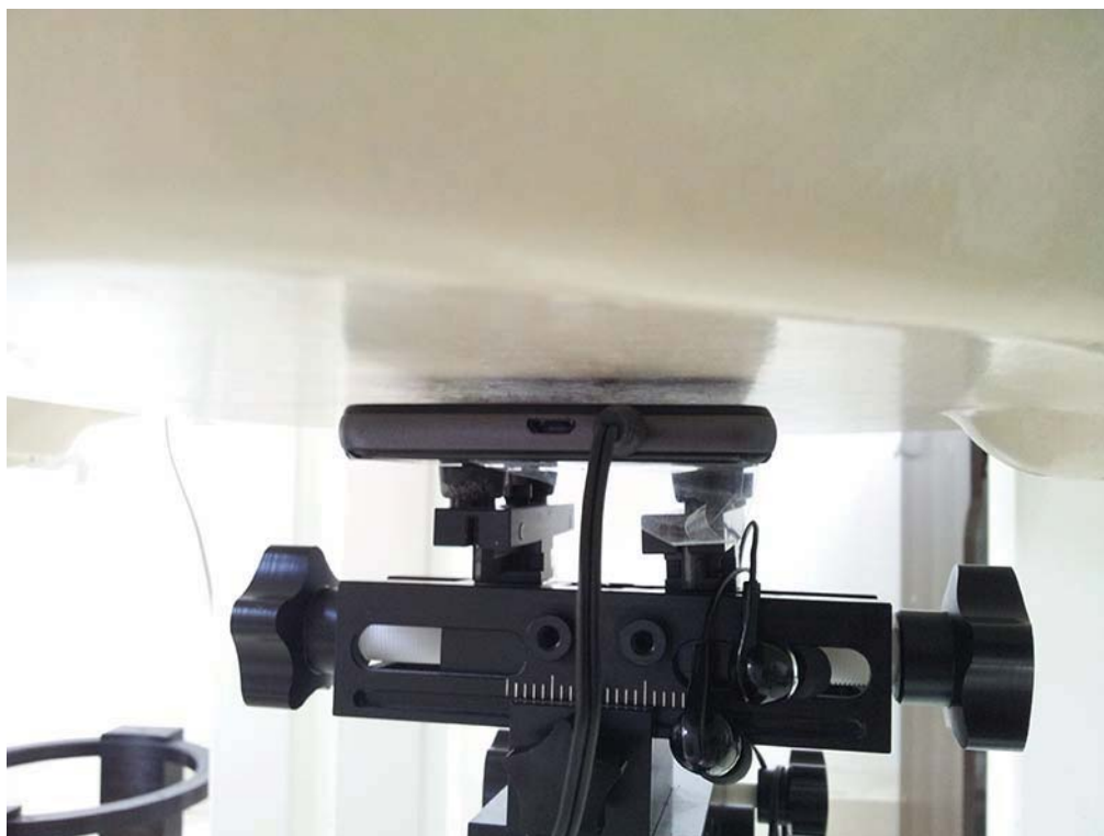
5mm Body-worn accessory with Headset Rear Side Setup Photo
