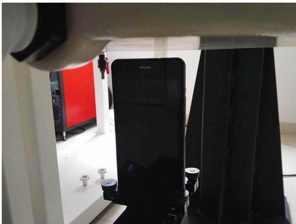
10mm Hotspot mode Top Side Setup Photo
