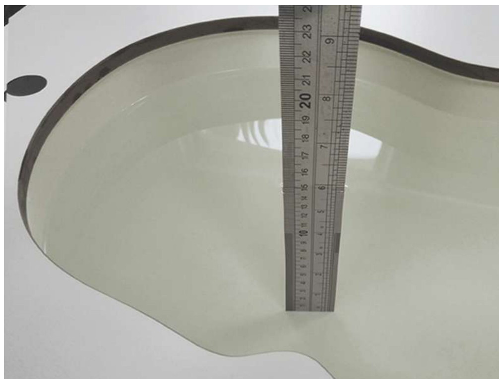
Liquid depth in the head Phantom (2450 MHz, 15.0cm depth)
