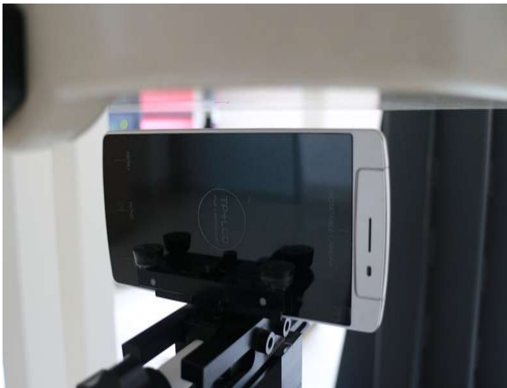
10mm Hotspot mode Left Edge Setup Photo
