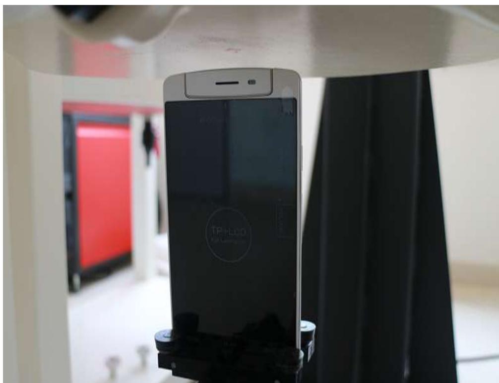
10mm Hotspot Mode Top Edge Setup Photo
