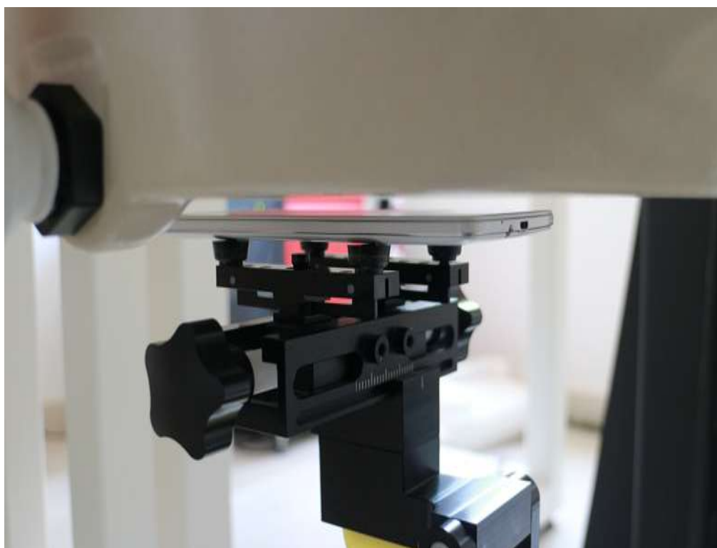
5mm Body-worn Accessory& Hotspot Mode Front Side Setup Photo
