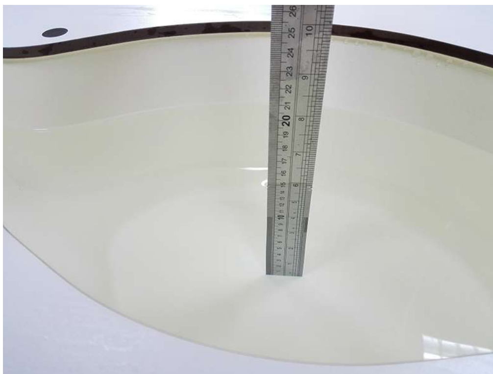
Liquid depth in the flat Phantom (1900 MHz, 15.2cm depth)
